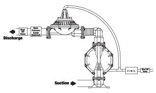
Proper support of piping and pulsation dampener is required.
