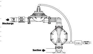
Proper support of piping and pulsation dampener is required.
