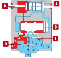
Diaphragm has pushed actuator pin (B) and Simul-Shift Valve (A) to the right.
