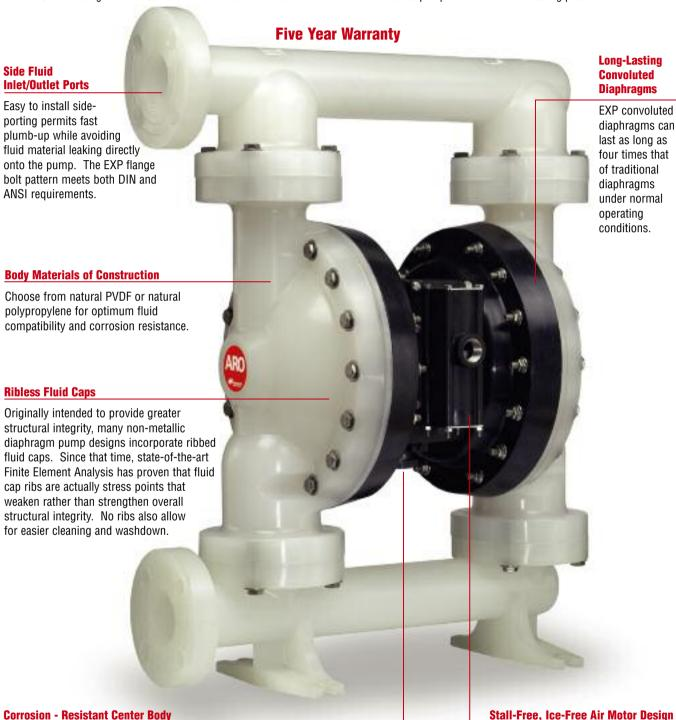
Non-Metallic Air Motor - Featuring a glassfilled polypropylene construction and thermoset vinyl ester, the EXP air motor is both strong and resistant to chemical attack.
