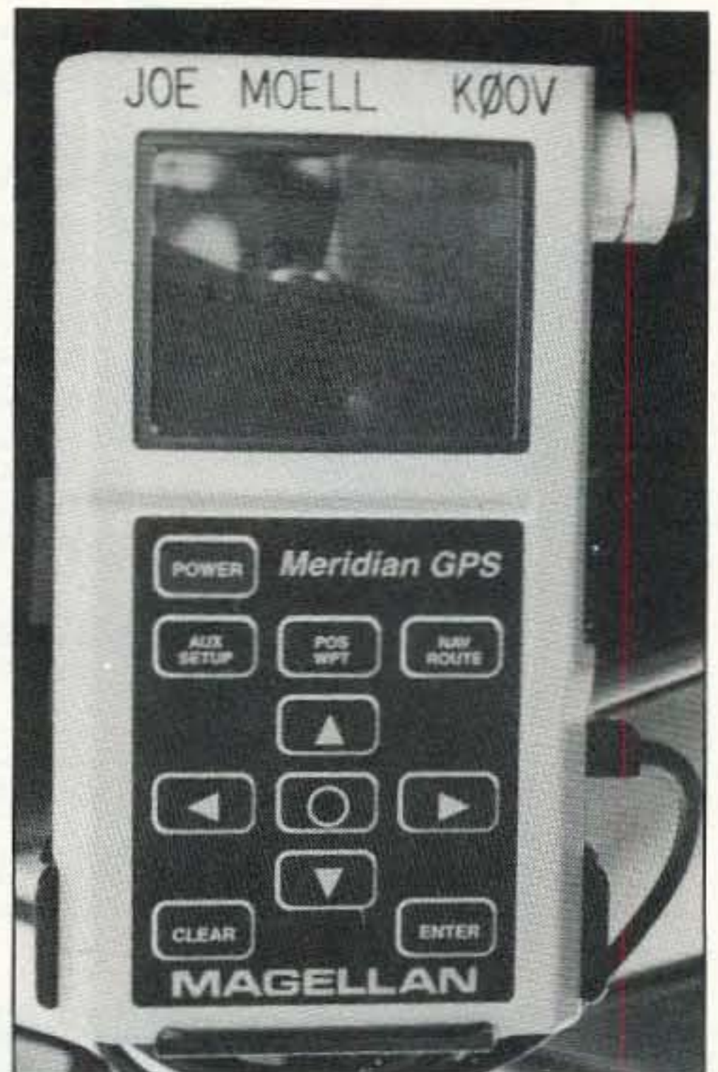
Photo A. I used a cellular phone swivel mount to attach the Magellan GPS bracket to the overhead console in the van to put it at eye level. A four-foot length of RG-58 cable connects it to the rooftop antenna.
