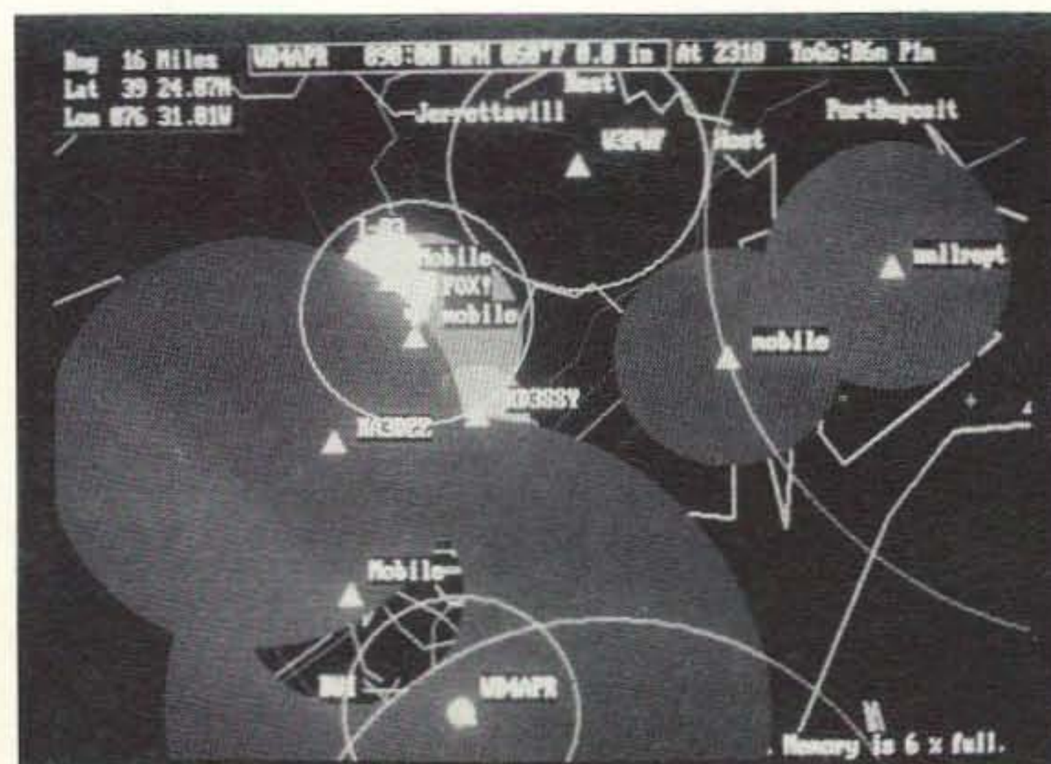
Photo D. APRS plots overlapping signal strength contours of reports from stations with omnidirectional antennas. The large (violet on the actual screen) circles show negative reports. Chances are, the hidden transmitter is not in those regions. Brighter, smaller circles in shades of blue on the screen show places where the fox signal is heard with various strengths.
