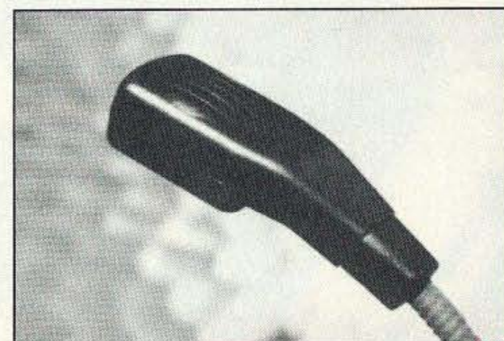
Photo B. The boom mike element is housed in a noise-cancelling enclosure.
