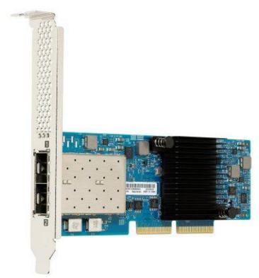
Figure 1. Emulex VFA5 ML2 Dual Port 10GbE SFP+ Adapter
