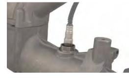
**RIVA EXHAUST** AIR/FUEL **RATIO SENSOR MOUNTS**
