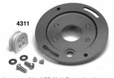
One of the advantages of the MSD Multi-Channel Ignition system is the individual trigger pickups for each cylinder. This way you can make up for the variations in fuel flow dynamics to each cylinder, exhaust characteristics or carb synchronization by altering the timing of each cylinder,
