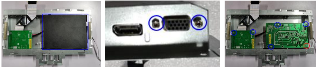
Separate screws from PCBA board
