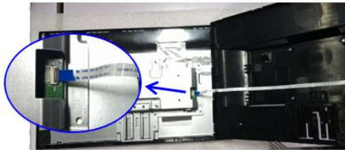
Separate the cable
