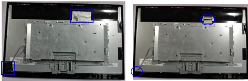
Separate taps and cable
