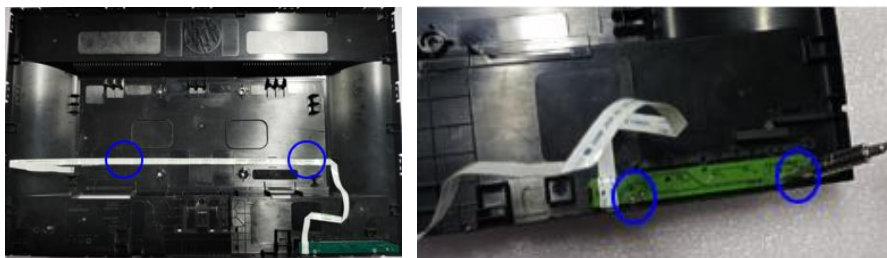
Separate keyboard from rear cover
