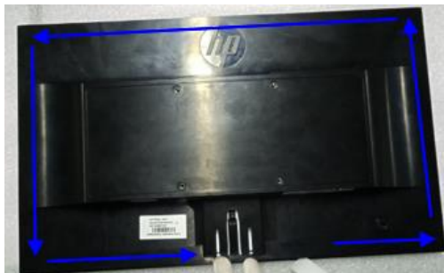
Separate the front bezel and rear case
