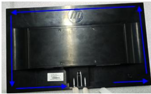
Separate the front bezel and rear case
