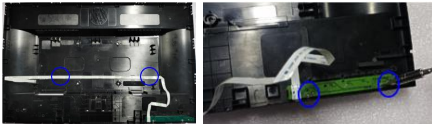
Separate keyboard from rear cover
