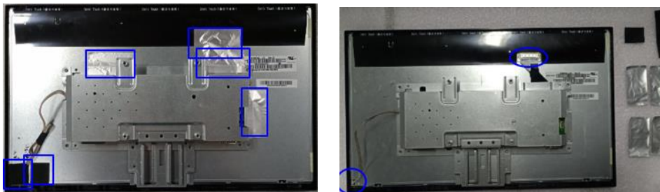
Separate taps and cable
