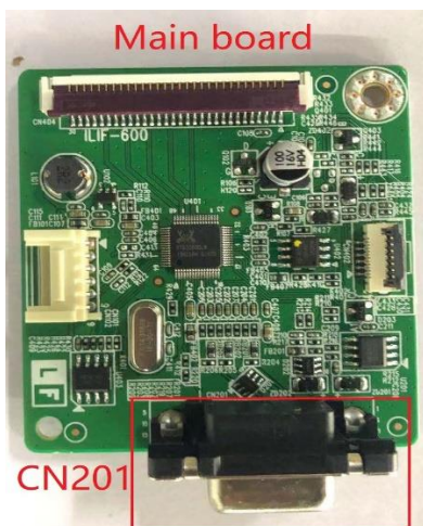
Connector location of Mainboard
