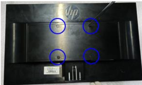
Remove the rear cover screws
