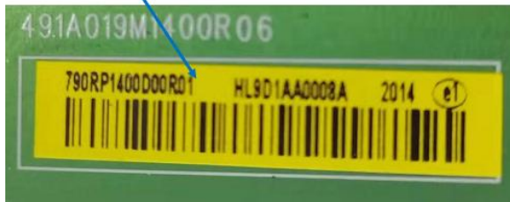
Part number location of power board
