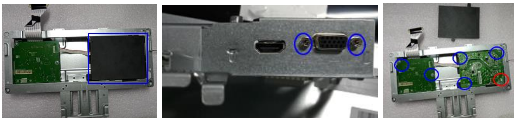
Separate screws from PCBA board
