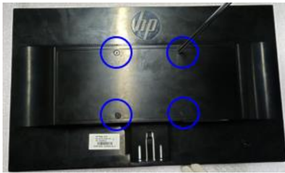
Remove the rear cover screws
