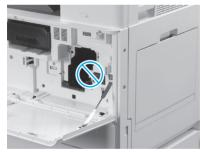
Ensure that the front and right doors are open. The right door retracts the interlock lever allowing the imaging unit to be installed.
