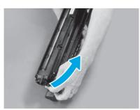
Remove the blue tab and tape from the imaging unit vent area.
