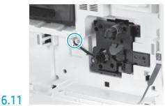
Connect the imaging unit connector to the engine connector.
