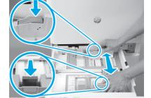
Push down on the blue tab in the back of the tray. At the same time, pinch or squeeze the blue tab in the front of the tray and slide to adjust to the proper paper length. Both tabs are spring-loaded and will lock, once released.
