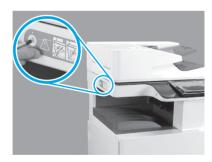
Remove the scanner lock screw and red sticker on the left side of the printer.  $\label{eq:printer} % \begin{subarray}{ll} \end{subarray} % \begi$
