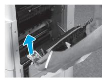
Open the right door and then remove the shipping label directing you to the transfer area.
