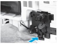
Slide the imaging unit into the device.
