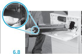
Hold the imaging unit with one hand on the bottom and the other hand on the gray handle at the front.
