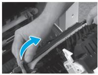
Carefully remove the strapping tape at the front of the transfer unit.
