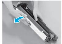
Remove white protective cover. Do not touch surface of the drum.
