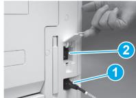
10.1 Connect the power cord to the printer and the wall
