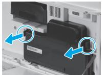
Push the latches on each side of the TCU and then remove the TCU.
