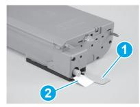
Remove two seals from the bottom and rear of the toner cartridge: Pull down to remove the seal on the bottom of the cartridge (callout 1). Pull out to remove the seal at the rear of the cartridge (callout 2).
