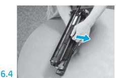
Pull straight out to remove the orange charge roller shipping lock.
