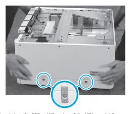
Lift and align the DCF or HCI on top of the HP LaserJet Spacer. Install two "L" shaped brackets and screws on the rear.
