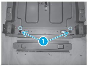
Remove two screws from the front support and remove. Install HCI front support with two screws. Move two sliver alignment pins (1) to new HCI support.
