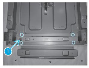
Remove four screws from the rear support and remove. Install HCI rear support with four screws. Move one sliver alignment pin (1) to new HCI support.
