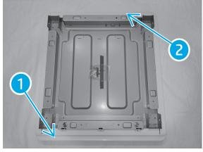
On the spacer remove six screws from the front (1) and rear (2) covers. Three are located on the outside and three more on the bottom. **NOTE**: You may need to loosen the rear side cover screws to release the rear cover.
