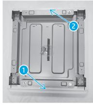
Reinstall Front and rear covers. Install four screws in each cover. If you had to loosen the side cover rears screws retighten them now.
