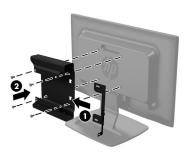
If mounting the sleeve to a ProDisplay monitor, remove the panel from the rear of the monitor. Place the 7mm spacer provided between the sleeve and the rear of the monitor ①, and then place the security bracket for your model into the rear of the sleeve so that it aligns with the screw holes on the sleeve and the padlock loop for your model ②. Attach the sleeve and spacer to the rear of a monitor using the 20mm machine screws provided ③.
