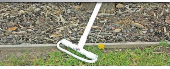
Wick Applicators are great for precision or drift free direct contact application, eliminating mist spray around valued plants or obstacles. Available as hand held Wick Stick for direct manual application or as a Boom Wick for vehicle attachment ideal for larger areas.
