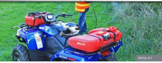
Silvan Quad Bike and Rakpak sprayers are designed to fit neatly on quad bikes and meet the strict weight requirement of these vehicles. The Wrap around design allows for a lower centre of gravity, essential for improved quad bike safety.
