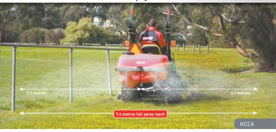
The Traylink sprayers eliminate the need for a PTO connection for small to medium boom spraying. The frames can be fitted to CAT 1 linkages, utilities, RTV's and trailers by only requiring a 12V connection for the high capacity pump. A boomless nozzle and spot spray qun are included.
