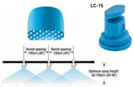
Nozzle can be mounted between 0" and ±90". Rotate nozzle bodies or raise or lower boom to attain 100% overlap of spray pattern. Ideal is +45" from level.
