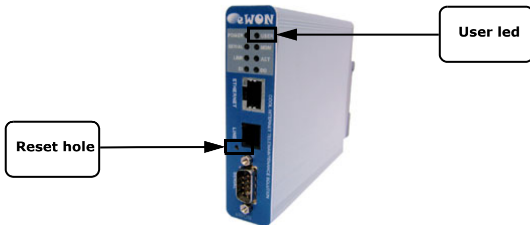
Figure 79: eWON - reset hole and "USER" led
