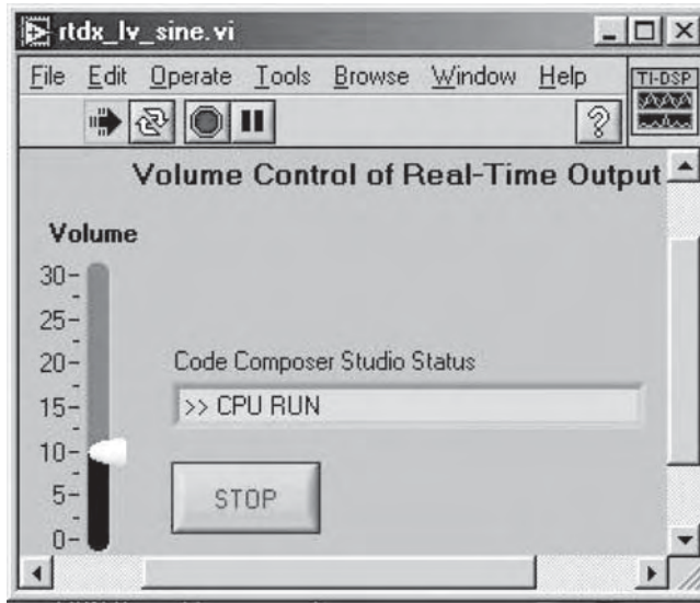
FIGURE 9.28. LabVIEW Instrument window for controlling the DSK output amplitude of a sine wave through RTDX for the project rtdx_lv_sine .
