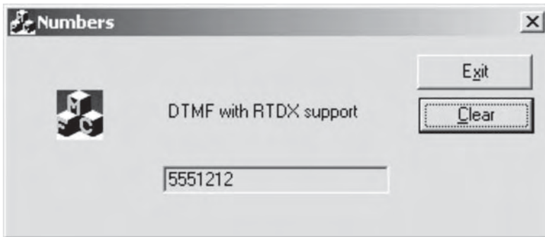
FIGURE 10.3. (a) Core C program to detect DTMF signals with RTDX for PC-DSK interface (dtmf_BIOS_RTDX.c); (b) PC screen displaying detected DTMF signals with RTDX for PC-DSK interface.
