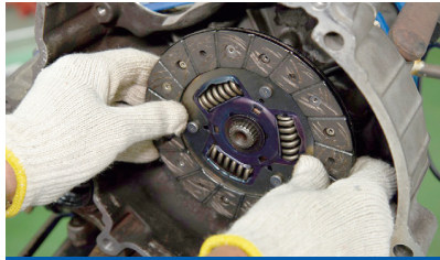
② Check for the Movement of Clutch
