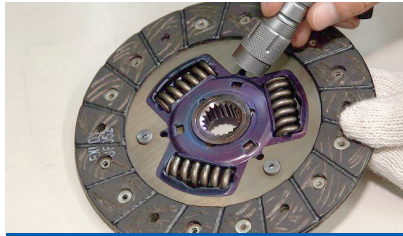
① Check for Clutch Disc Appearance
