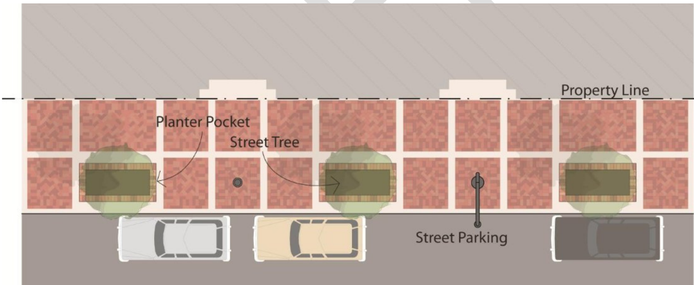
Figure 8: Planter Pocket Detail
