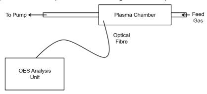
Figure 13: Schematic of OES apparatus.
