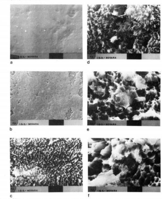
Figure 3. SEM results: (a) untreated sample; (b) after 1 min; (c) 2 min; (d) 5 min; (e) 10 min; (f) 15 min.
