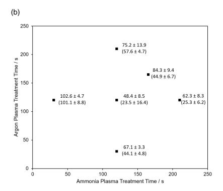
Figure 24: Average WCA achieved for samples in the (a) glow plasma region and (b) remote plasma region using different treatment time combinations of argon and ammonia plasma treatment (20 W, 30–210 s Ar plasma treatment, then 5 W, 30–210 s NH $_3$  plasma treatment, both at 0.2 mbar) after solvent washing (1:1 v/v solution propan-2-ol:cyclohexane, 10 s). Numbers in brackets correspond to the average WCA achieved prior to solvent washing. Errors shown are the standard deviation of the sample.
