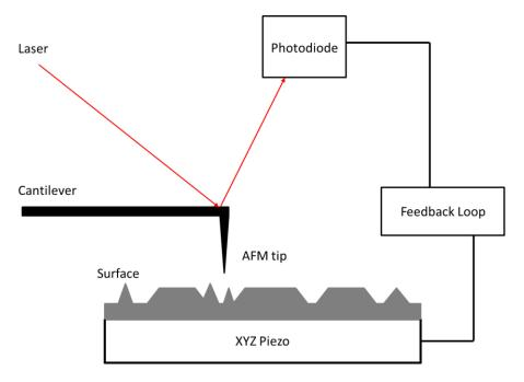
Figure 14: Schematic of AFM apparatus. As the sharp tip moves across the features of the surface, the cantilever angle moves slightly. The deflection angle is measured by the degree of deflection of the laser as it hits the photodiode. This is fed into the feedback loop which controls the XYZ piezo and the height of the surface in comparison to the AFM tip.
