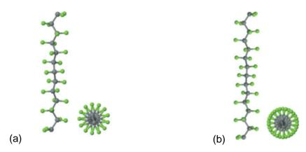
Figure 1: Molecular structure of PTFE. Pendant groups are arranged in a helical structure in order to minimise interactions. (a) Below 19 °C, the H-136 form is adopted by PTFE chains. (b) At room temperature, PTFE is arranged in the H-157 structure. Images adapted from article by C. Wang *et al.*<sup>6</sup>
