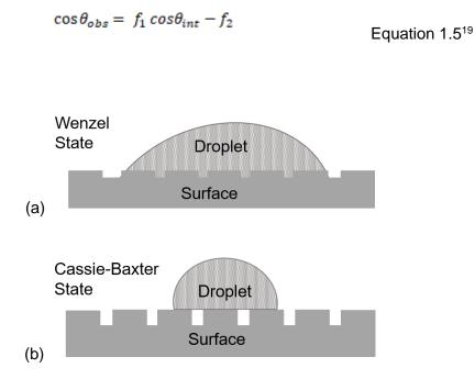
Figure 6: Wetting states of a surface. Schematic (a) depicts the Wenzel wetting state whereby the droplet permeates into the roughness of a surface, causing a decrease in observed contact angle. Schematic (b) shows the Cassie-Baxter state where air pockets are trapped in the surface roughness between the surface and the droplet. The result of which is an increase in the observed contact angle of the droplet with the surface.
