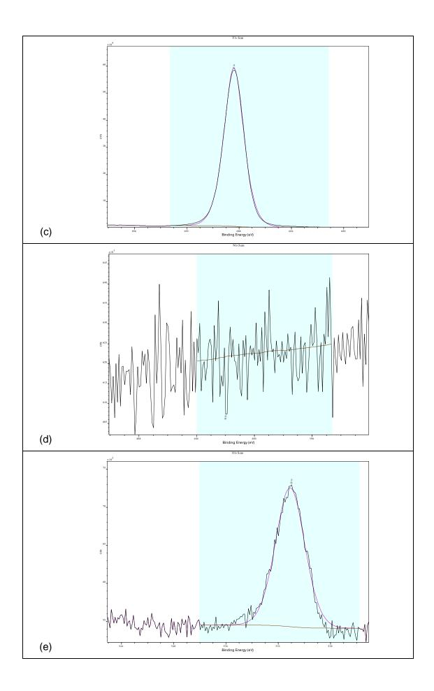
Figure 33: XPS of untreated washed Goodfellow PTFE. (a) Survey spectra; (b) C 1s high resolution scan; (c) F 1s high resolution scan; (d) N 1s high resolution scan; and (e) O 1s high resolution scan.
