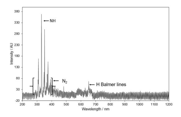
Figure 22: OES of  $NH_3$  plasma (50 W, 5 mins, 0.2 mbar). Labelled are the significant peaks as labelled in  $NH_3$  OES by S. Kang *et al.*<sup>202</sup>
