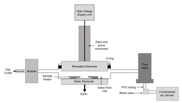
Figure 42: Schematic representation of DBD apparatus with flow meter allowing for constant flow of air through the flow cell.
