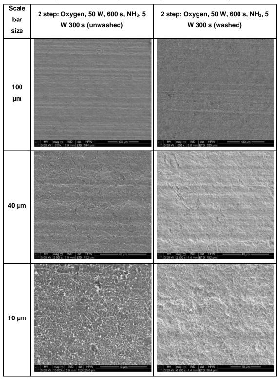
From Table 21, it is clear that the effect of solvent washing on the two-step plasma-treated surfaces is the removal of the submicron size white debris from the surface. This coupled with the observed increase in WCA (Table 18) after solvent washing would indicate that the effect of the solvent wash is to remove LMWOS species from the surface. Through the analysis of the wash liquor, the identity of these species may be further investigated.
