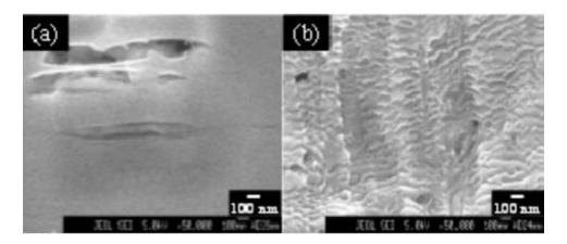
Figure 18: FE-SEM images at 50 000 magnification and 5.0 kV electron acceleration voltage of PTFE (a) as received, WCA 118°, and (b) treated with Ar/NH<sub>3</sub>-H<sub>2</sub>O plasma (100 W, 15 min, 0.8 mbar), WCA 4°.<sup>147</sup>
