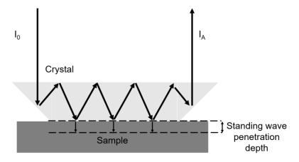
Figure 15: Total internal reflection of  $I_0$  within the Diamond cut KSR-5 (thallium bromoiodide) crystal, and the resultant standing wave that penetrates the sample. Adapted from schematic by S. Morsch.<sup>89</sup>
