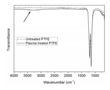
Figure 29: FTIR-ATR (Nicolet iS10, Thermo Scientific, fitted with ATR sampling accessory (Smart iTR), 32 scans and a resolution of 2 cm<sup>-1</sup>) spectra of untreated and oxygen plasmatreated PTFE (200 W, 600 s, 0.09 mbar). Arrow points to region where the OH containing bands are present.<sup>176</sup>
