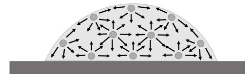
Figure 2: Surface tension of a droplet of liquid on a surface. The interfacial molecules have an imbalance of forces compared the bulk and so the droplet contracts to minimize the surface free energy. Based on schematic by Y. Yuan and T.R. Lee. <sup>17</sup>
