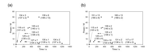
Figure 27: Average WCA achieved for samples in the (a) glow plasma region and (b) remote plasma region using different treatment time combinations of oxygen plasma treatment (2–50 W, 75–1200 s, 0.2 mbar) after solvent washing (1:1 v/v solution propan-2-ol:cyclohexane, 10 s or 2min). Numbers in brackets correspond to the average WCA achieved prior to solvent washing. Errors shown are the standard deviation of the sample.
