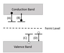
Figure 36: The processes by which charge is incorporated into an insulating surface. (A) An electron drops from the bottom energy level of the conduction band, known as electron trapping. (B) An electron is promoted into the conduction band, termed electron releasing. (C) Hole promoted from the top energy level of the valence band, known as hole trapping. (D) Hole drops down to the top level of the valence band, termed hole releasing.<sup>283</sup>
