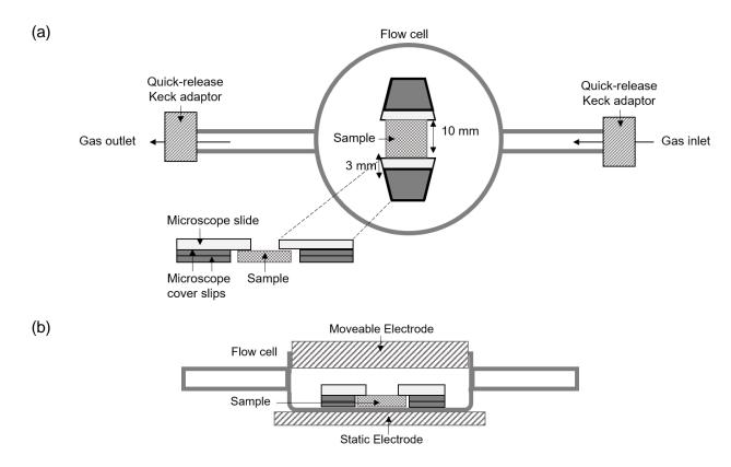
Figure 41: Sample holder and glass flow cell. (a) Top-down view and sample holder blow-out. (b) Side view of flow cell. The moveable electrode had no dielectric material.
