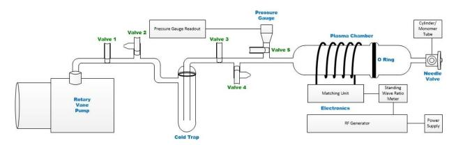
Figure 19: Schematic representation of low-pressure plasma reactor. Created by James Wigzell and reproduced with thanks.
