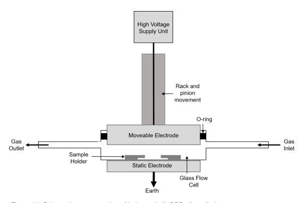
Figure 38: Schematic representation of in-house built DBD silent discharge apparatus.
