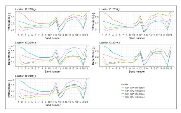
Figure 5.1: Atmospheric correction of S3A and S3B OLCI bands for coordinates of interest
