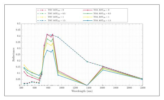
Figure 5.8: Response of SPART model with varying AOT values
