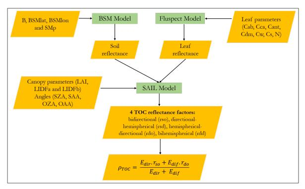
Figure 2.1: Structure of the forward radiative transfer of incident radiation in the SCOPE model (BSM, Fluspect and RTMo).
