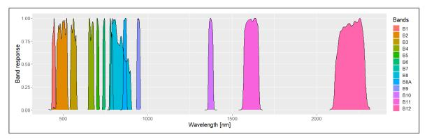
Figure 3.3: Spectral response functions of Sentinel-2 MSI bands
