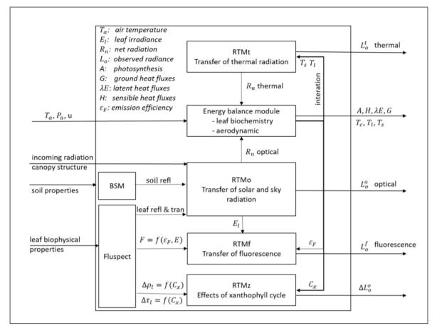
Figure 2.3: Structure of the SCOPE model (from Yang, Prikaziuk et al., 2020)
