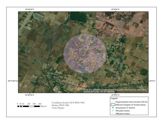
Figure 4.2: Effective ground footprint (blue polygon) of Sentinel-3 OLCI dataset, expected ground footprint (transparent pink polygon) and S3A (magenta dots) and S3B (yellow dots) pixel centres.
