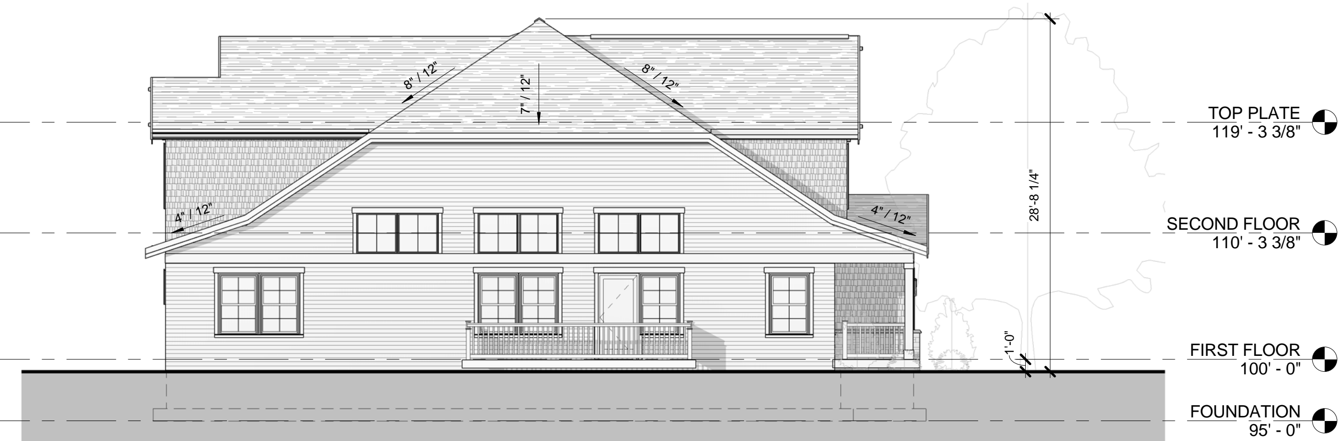
C6 ELEVATION - PROJECT WEST 1/8" = 1'-0"
