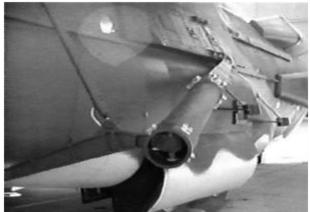
USAF Photo Eight Mark 56 rocket motors (four on each side) were mounted on the aft rear fuselage area and were pointed rearward at a 45-degree angle.
