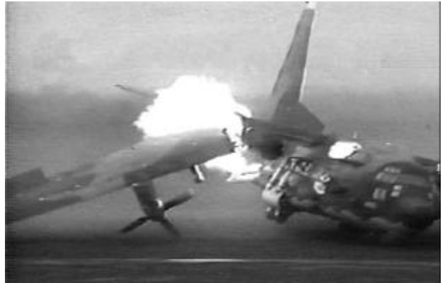
USAF Photo With all eight ASROC rockets fired, the aircraft's forward flight vector was reduced to near zero, resulting in rapid descent to the runway. The right wing broke between the number three and number four engines. The aircraft is traveling down the runway just after impact.
