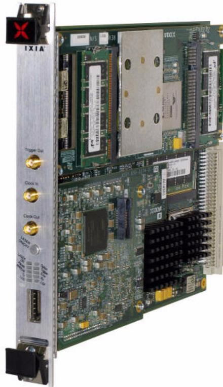
**Note.** Due to power requirements, only one MSM module can be used in a 250 or 400T chassis. Other modules can be used with the MSM in the same chassis, but only one CPM1000T8 at a time (except the CMP1000T8 module, which has the same limitation).
