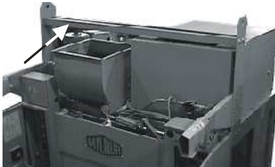
Figure 3: Spreader Bar Between Front Lifting Plates
