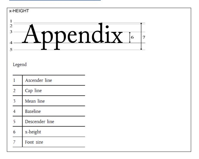
The X-height is provided in line 6. In general, this should be minimally 1.2 mm (see above articles).
