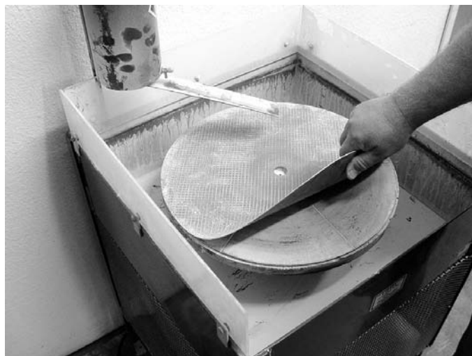
Shown above is Magnetic Nova being removed from an 18RL lap machine.
