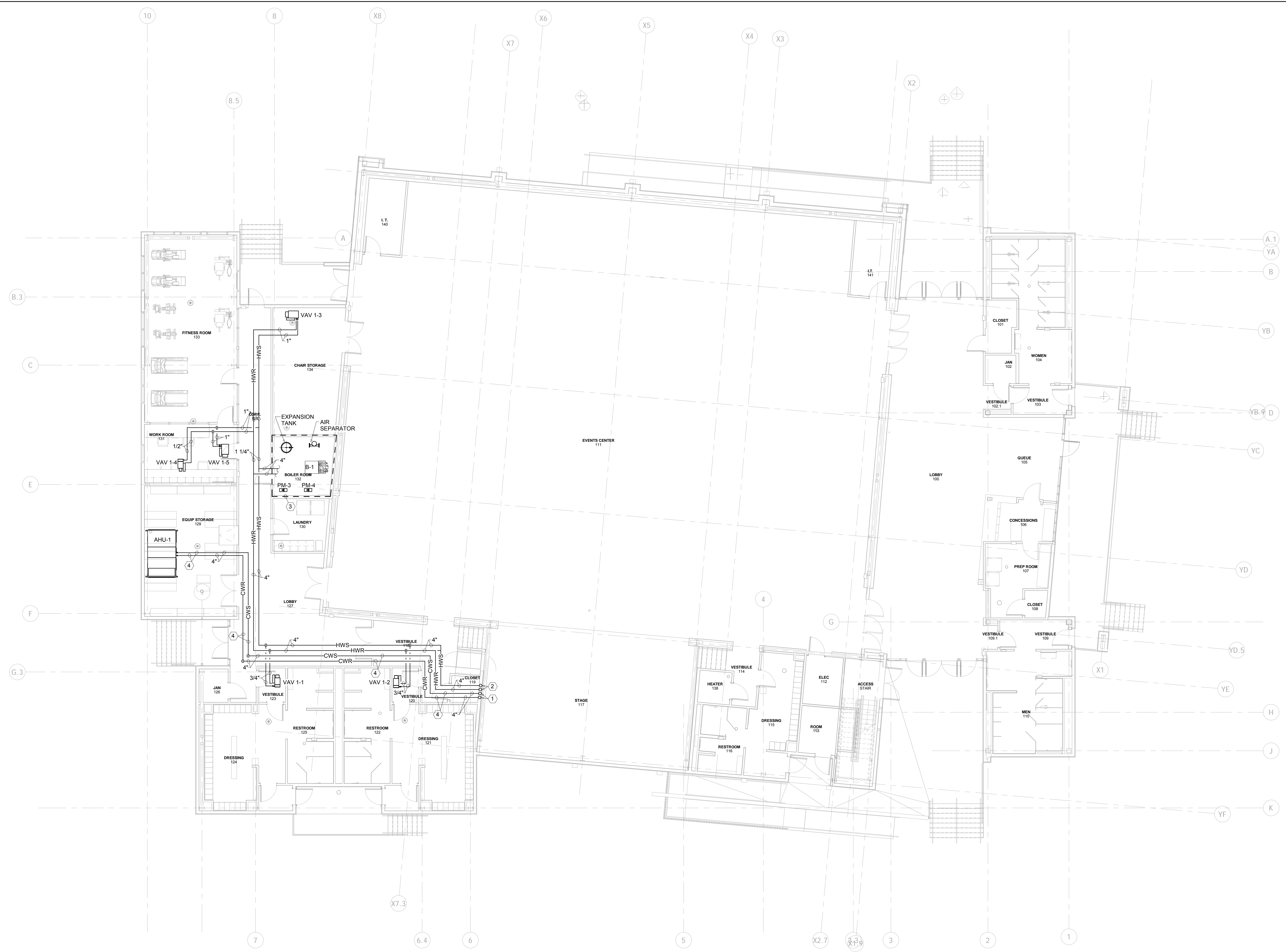
1 M201 FIRST FLOOR PLAN - HYDRONIC PIPING 1/8" = 1'-0"
