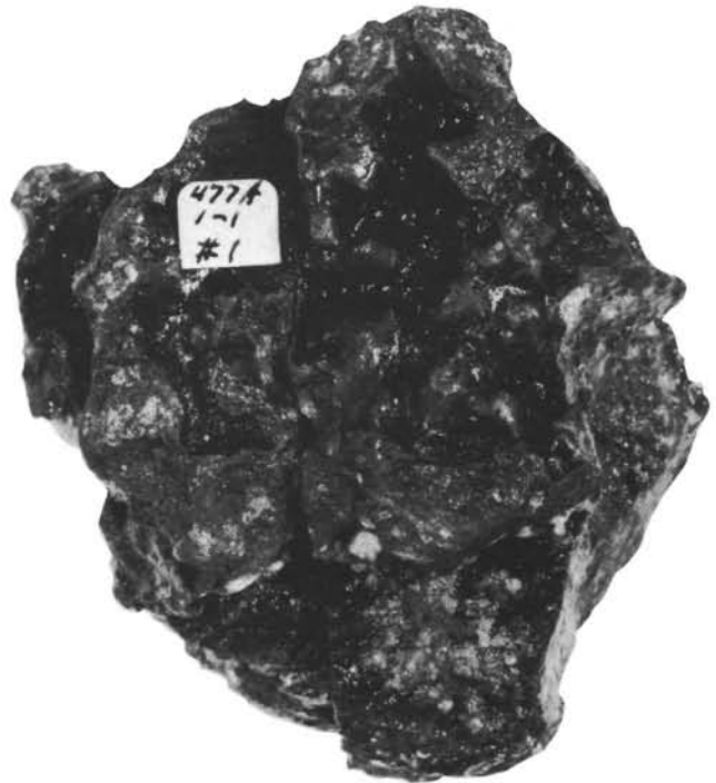
Figure 22. Section 477A-1-1, Piece 1. Upper chill margin from doleritic sill.
