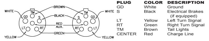
NOTE: Identify contacts by looking into the open end of plug or socket.
