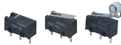
Body : H=6.5, W=5.8, D=12.8, Fixing centres=5.08 Actuator lever L=12.8
