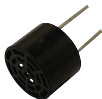
Body - Dia. = 9.9, H = 7.1mm Pins - Dia. = 0.64, L = 10mm
