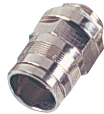
Panel housing and locknut D(front panel)=36, L=42, Panel thickness=4 max Panel cut-out=21 Thread=Pg13.5
