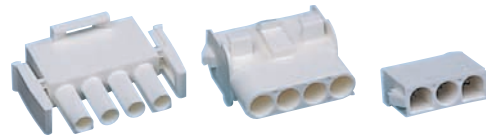
Plug housing Mates with receptacle or PCB header Cable or panel Mounting receptacle Panel thickness = 0.76-2.29 PCB Header PCB hole dia. = 1.8 Pitch = 6.35
