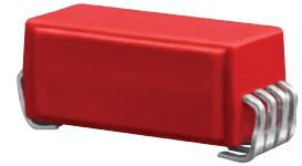
Model 9802 J-Lead - No shield fitted Gull wing - H = 4.31, W = 11.68, D = 4.95mm J-Lead - H = 4.82, W = 11.18, D = 4.95mm
