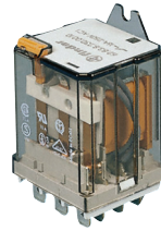
H (case) = 48, H (incl. fixing lugs) = 68, W = 38.2, D = 35.8 Fixing centres = 63.5, Slot W = 3.6, Terminals Faston 250 = 6.35 x 0.8
