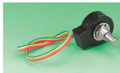
Ribbon Cable Horizontal PCB Vertical PCB Shaft=22 (incl. bush), dia.=6.35 Mounting bush=3/8" x 32 NEF Ribbon cable length=190
