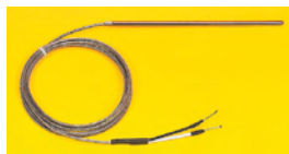
Probe L = 150, Dia = 4.76, Lead L = 2mx7/0.2
