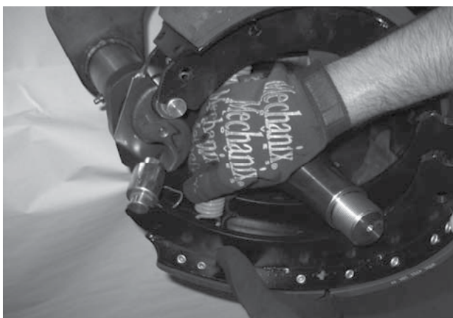
Figure 47. Removal of Return Spring
