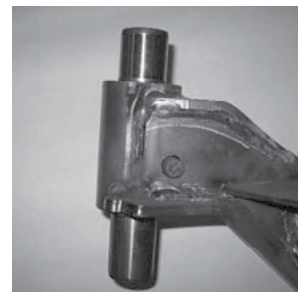
Figure 22. Kingpin After Cleaning
