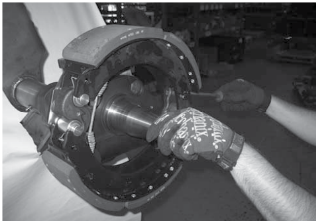
Figure 46. Removal of Outer and Inner Retaining Spring
