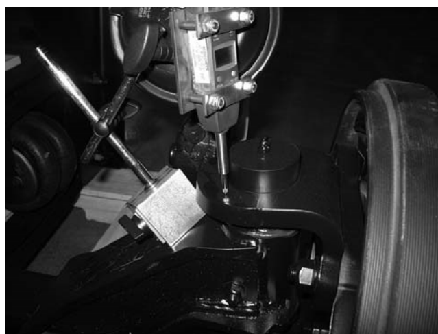
Figure 6 Vertical End Play Checking
