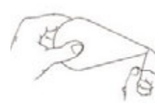
Label dispenses automatically when the liner is pulled from the front of the unit.
