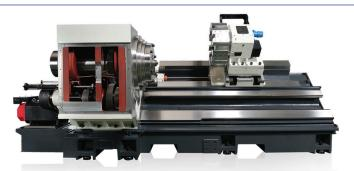
**Turret:** Massive, 7.7" thick disk and hydraulic clamping of its curvic-coupling design ensure cutting stability during rough-turning environments. Live tooling max. speed is 3,000rpm/ power is 15 HP.
