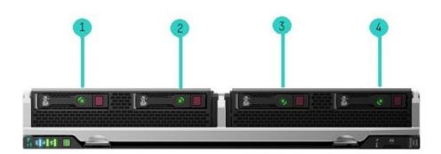
1-4 4 x SFF hot-plug drive bays for SAS, SATA, SAS SDD, SATA SSD, NVMe PCle SSD, or up to 8 uFF with Smart Drive Carrier adapter
