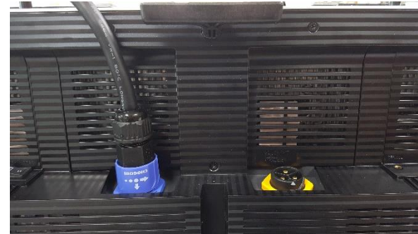
② Connect the other end of Power Daisy Chain Cable to the Input Power Connector of next cabinet.
