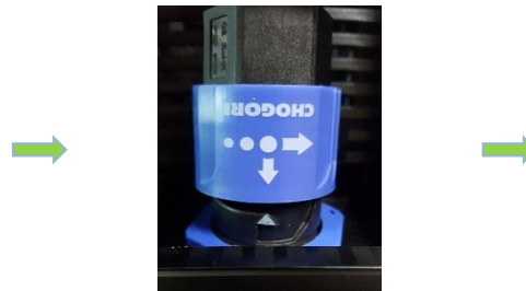
② Insert the cable into the Cabinet DC Inlet to meet the two arrows.
