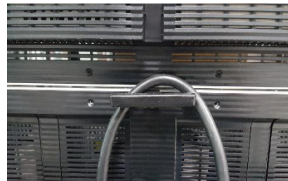
⑤ To protect the connectors from damage or stress caused from the heavy weight, hang on the cables on the handles of cabinets like the upward.
