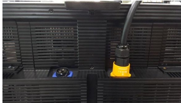
① Connect the Power Daisy Chain Cable to the Cabinet Output Power Connector. (Input – Blue, Output – Yellow)
