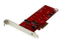
This M.2 SSD controller card lets you install two M.2 SATA solid-state drives (SSD) into your PC through PCI Express. You can mount virtually any M.2 drive directly to the card, giving you a convenient and discreet way to improve your computer system performance.
