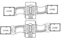
**NOTE:** Only one Source disk and one Destination disk can be installed at a time. Only connect a SATA or an IDE hard drive, not both.
