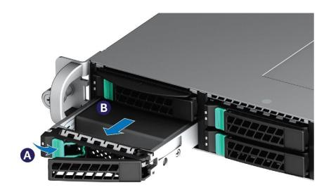
Figure 30. Hot Swap Storage Device Carrier Removal
