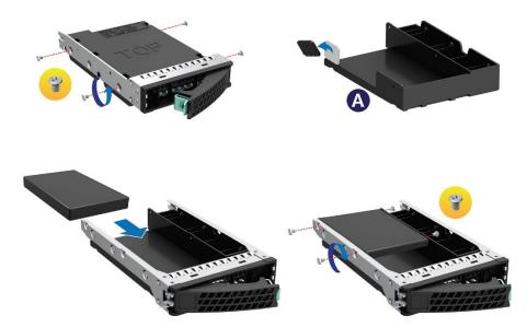
Figure 31. 2.5" SSD mounted to 3.5" Drive Tray
