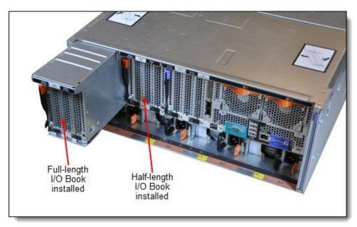
Figure 12. I/O Books that are installed in the x3850 X6
