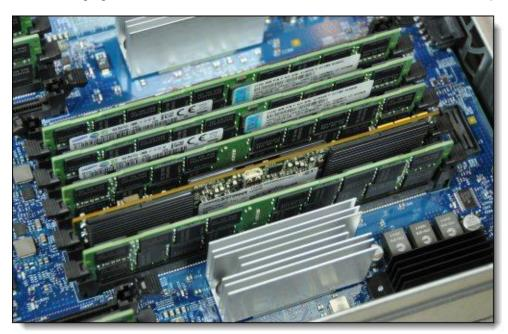
Figure 5. IBM eXFlash DIMM installed in the Compute Book
