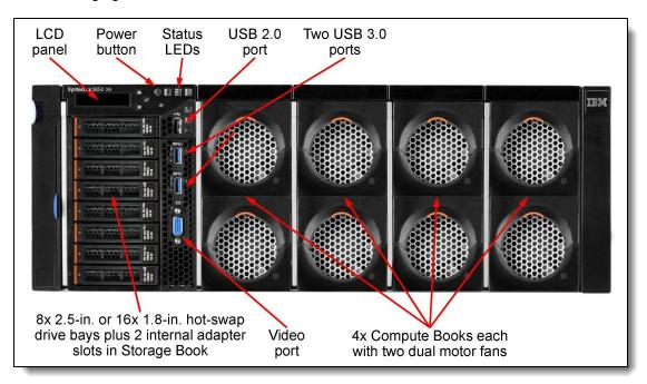
Figure 2. Front view of the IBM System x3850 X6
