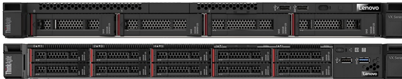
Figure 1. Lenovo ThinkAgile VX 1U Certified Node with 4x LFF (top) or 10x SFF (bottom) drive bays
