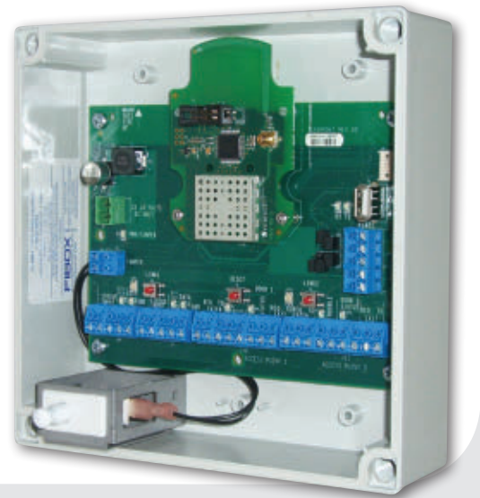
Networked Locking Solutions PIM400-TD2 Panel Interface Module
