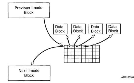
Figure 1-3. Direct Pointers from an I-node to Data Blocks
