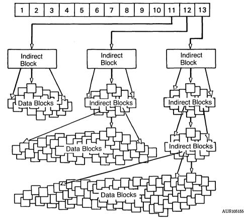
or 2,113,674 blocks. Figure 1-4 shows the relationship of data blocks and indirect blocks associated with an i-node.
