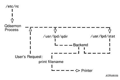
Figure 3-1. How the Queueing System Works
