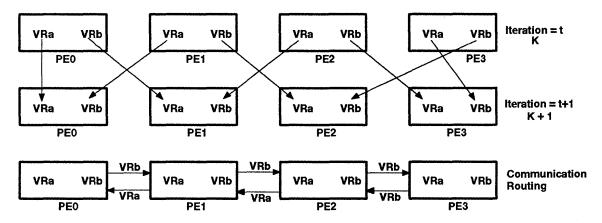
Figure 5. Parallel Jaccobi Updating on a Systolic Architecture
