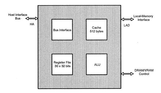
The TMS34020 unique memory interface speeds performance of tasks such as bit alignment and masking while supporting advanced DRAM access modes. The 32-bit architectures supplies the large blocks of contiguously-addressable memory that are necessary in graphics applications.
