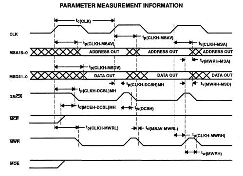
NOTE: This example shows multiple data writes. Timing for multiple code writes would be similar. This option for using DS/CS as data space chip enable and MCE as code space chip enable is invoked by setting the MEMCFG bit high in the configuration register. When MEMCFG is high, DS/CS and MCE rise after every rising clock edge. In this mode, DS/CS and MCE may not both be active (low) at the same time.
