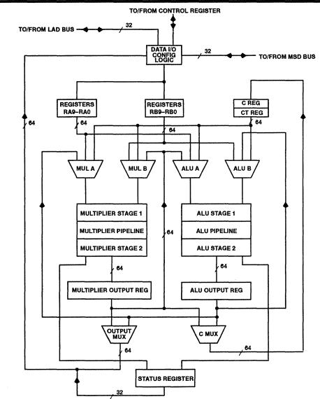
Figure 8. FPU Core Functional Block Diagram
