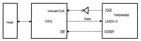
The TMS34082 only drives the LAD bus during instructions that output an address or data. The LAD bus drivers are disabled at any other time.
