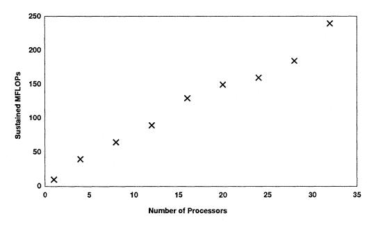
Figure 7. 128 x 128 Matrix Multiplication on P-Processor Systems
