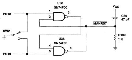
Figure 26. TMS34082, Details of U38
