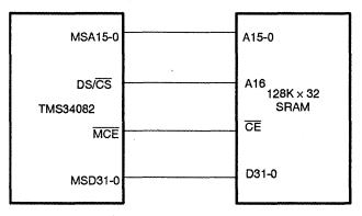
When MEMCFG is high,  $\overline{\text{MCE}}$  becomes the code space chip enable and DS/ $\overline{\text{CS}}$  the data space chip enable. Both are active low. This may eliminate the need for an external inverter on DS/ $\overline{\text{CS}}$ . Figure 4–8 show this configuration.
