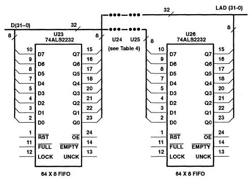
Figure 21. FIFO Logic, Details of U23, U24, U25, and U26
