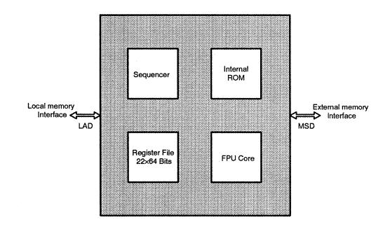
The TMS34082 complies fully with IEEE Std 754-1985, the industry standard for binary floating-point formats. Floating-point operands can be either singleor double-precision. In addition to floating-point operations, the TMS34082 performs 32-bit integer arithmetic, logical comparisons, and shifts. Integer operations may be performed on 32-bit 2s complement or unsigned operands. Floating-point to integer and integer to floating-point conversions are also available.
