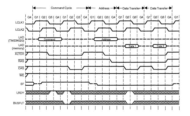
Figure 5–6. Transferring Memory to the TMS34082
