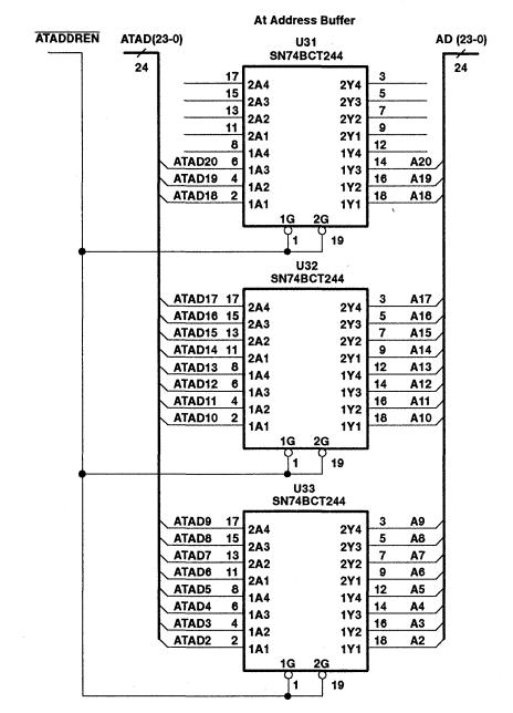
Figure 12. Motorola MC68030 and Address Buffers, Details of U31, U32, and U33
