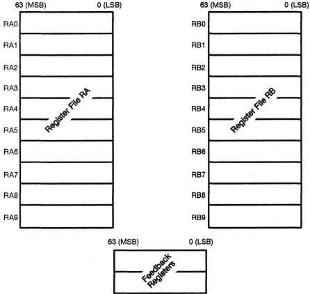
When the ONEFILE control bit is set high in the configuration register, data written to a register in RA file is simultaneously written to the corresponding location in RB file. For example, the same data is written to both RA1 and RB1 at once. In this mode the two register files act as a ten-word, two-read/one-write register file, as shown in Figure 4–5.
