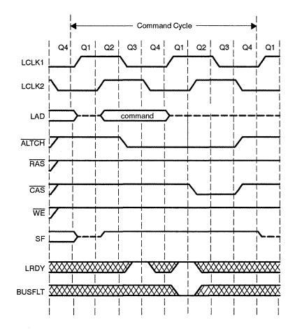
Figure 5–3. Transferring a Command from the TMS34020 to the TMS34082
