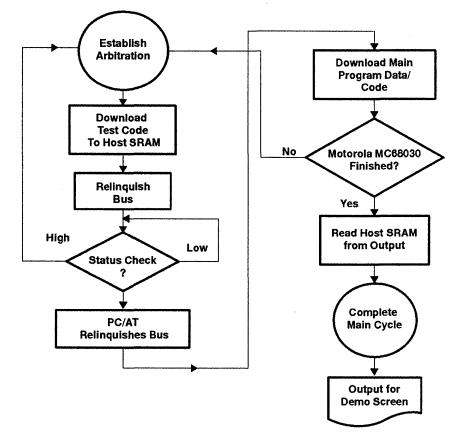
Figure 5. Block Diagram – PC/AT Code
