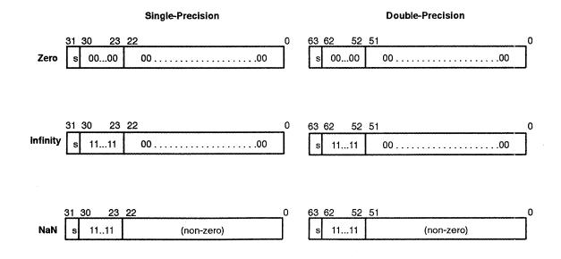
Figure 3–5. Special Floating-Point Formats
