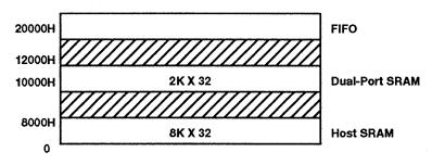
Figure 7. Motorola MC68030 Interface: Memory Addressing
