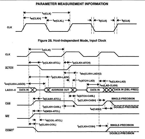
† COINT timing is for LADCFG high only. When the LADCFG bit is set high in the configuratin register, COINT is controlled by bit 1 of the LAD move instruction instead of the set mask instruction.
