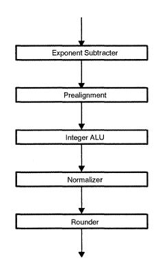
Integer processing in the ALU includes both arithmetic and logical operations in either 2s complement numbers or unsigned integers. The ALU performs addition, subtraction, comparison, logical shifts, logical AND, logical OR, and logical XOR. Format conversions and wrapping/unwrapping of denormals are also done by the ALU.
