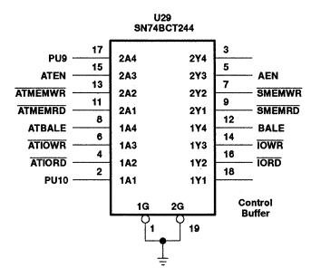
Figure 10. PC/AT I/F and Control, Details of U29
