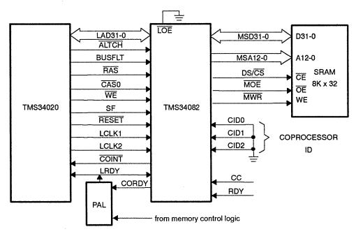
The maximum amount of external memory directly addressable by the TMS34082 is 64K words of program code and 64K words of data as shown in Figure 5–13. This comes out to 512K bytes total. When additional memory is necessary, segmentation or paging techniques can be utilized.
