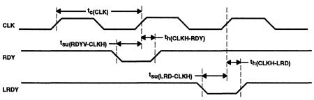
NOTE: When either RDY or LRDY is set low and the setup time before CLK high is observed, the device is stalled for one or more clock cycles, until RDY or LRDY is set high again. During a wait state, internal states and status are preserved and output signals do not change. LRDY can be used in this manner only in the host-independent mode.
