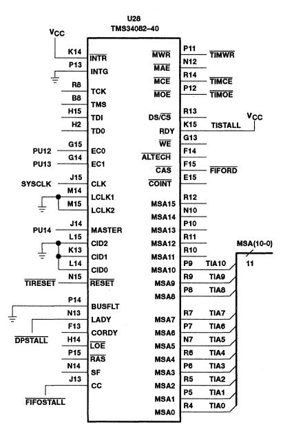
Figure 28. TMS34082, Details of U28
