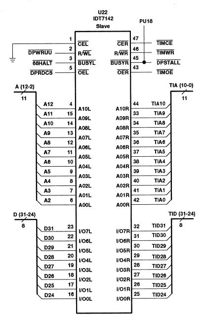
Figure 24. FIFO Logic DP-SRAM, Details of U22
