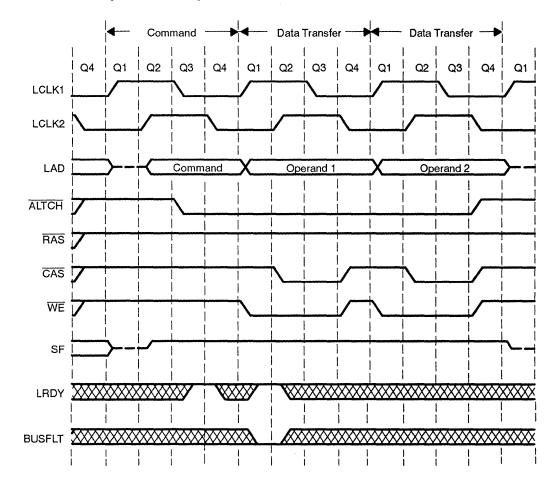
Figure 5-4. Transferring TMS34020 Registers to the TMS34082
