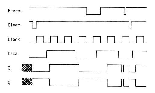
Shown below is a timing diagram for a D flip-flop.
