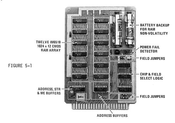
The board is fully nonvolatile using penlite chips to retain the RAM chips in the low power data retention mode. Thus, the user may write programs on a board, unplug it and use a different board without losing programs. The board may be mapped into memory space according to several jumper options. The board may also be configured as either an Instruction Field or a Data Field by jumper option. (Refer to the IM6100 brochure and Applications Bulletin M007)
