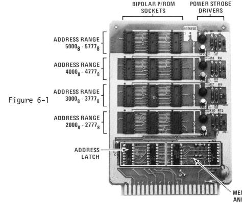
MEMORY ENABLE AND POWER STROBE DECODING LOGIC
