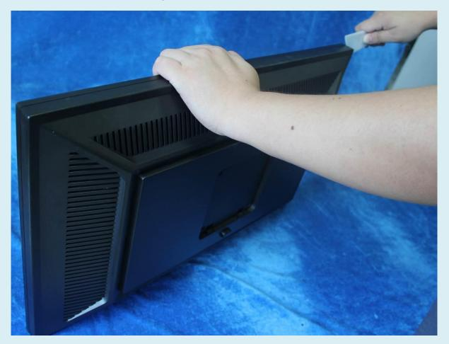
Note: The positions of the clips on the rear cover are as follow. There are some small gaps between CLIPS. It's suggested to separate bezel and rear cover from the gaps.
