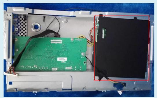
And then remove screws in red, pull out the wire to remove the main board and power board.
