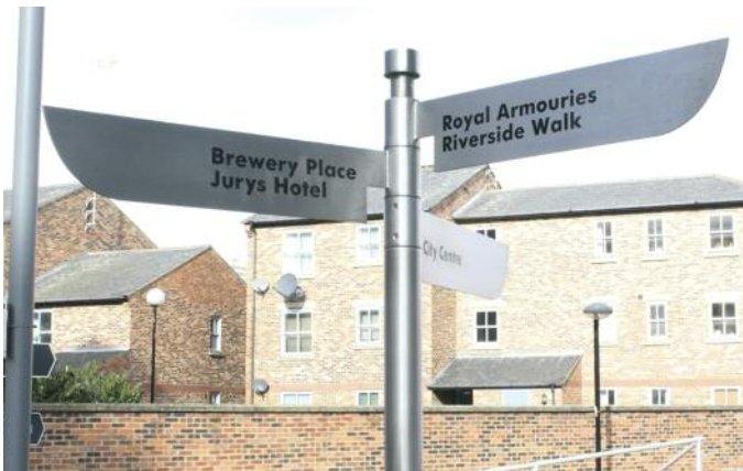
The classic cast aluminium or iron finger post has been given a modern interpretation using stainless steel with etched and painted letters at Brewery Wharf, Leeds.
