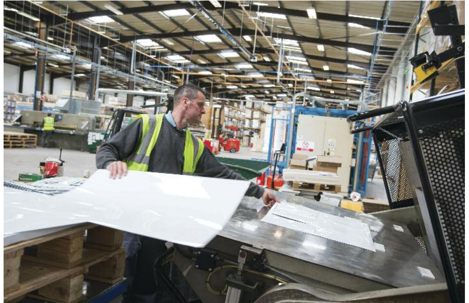
Die cutting inside the new specifically converted warehouse and office in Leeds.
