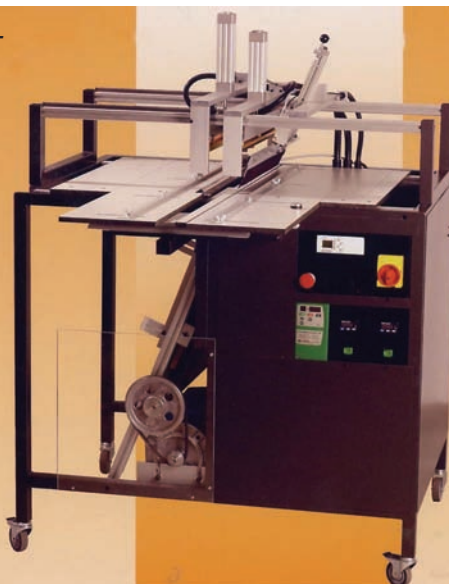
The FBM is a semi-automatic folding machine
