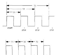
This article will use the SYM-1 board's 6532 timer and keyboard display to create a device which can measure up to 50 time intervals, store them in memory and then read them out one at a time.
