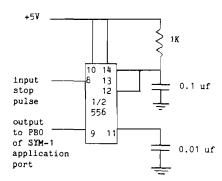
Figure 3: Connecting a 556 timer for use as an interface to the event timer.
