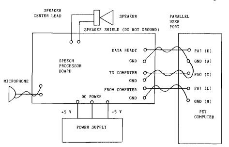
Figure 1: Speech processor components
