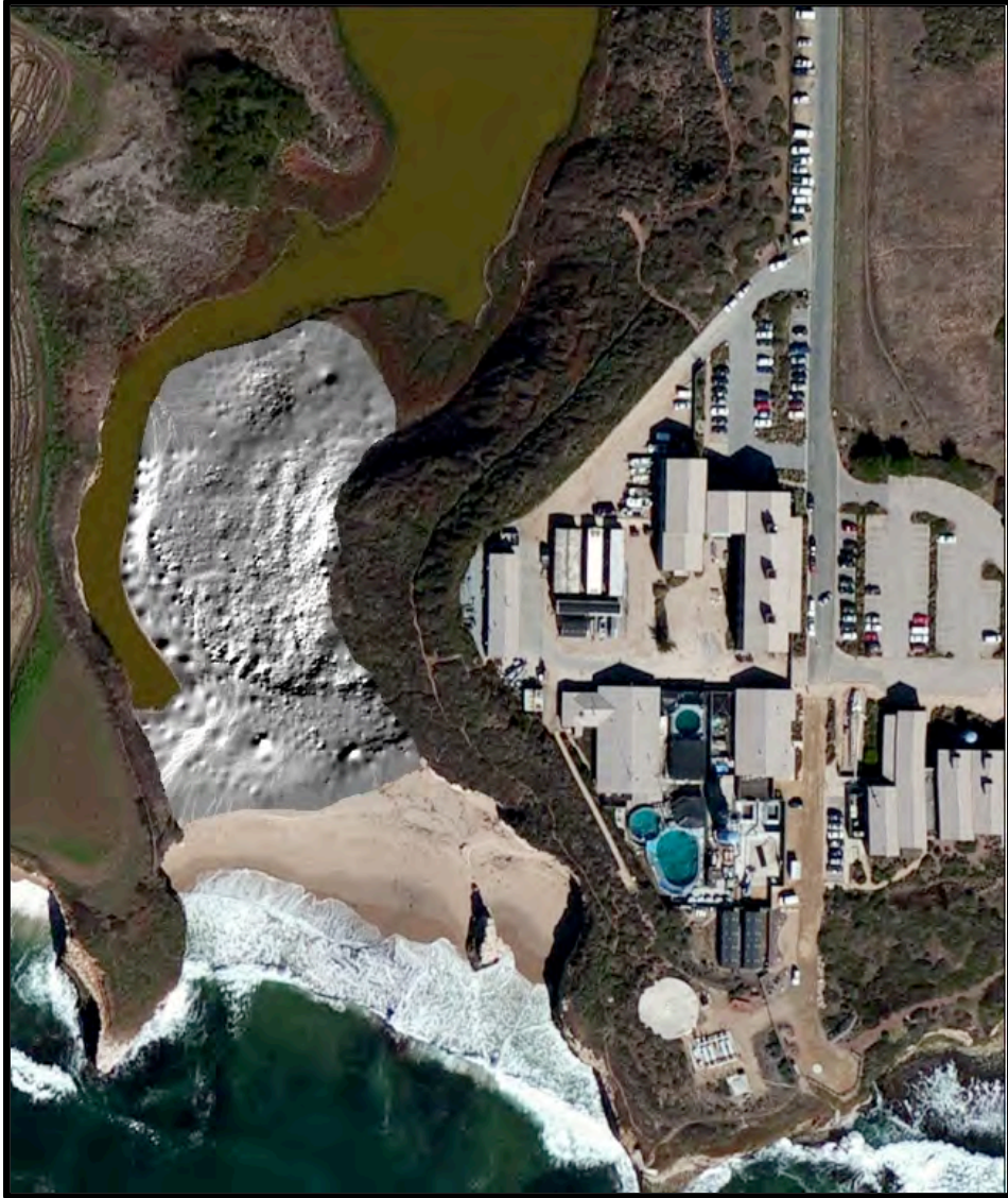
Figure 9. Younger Lagoon dune map. Survey data and resulting elevation model output shows topographic features on Younger Lagoon Beach.
