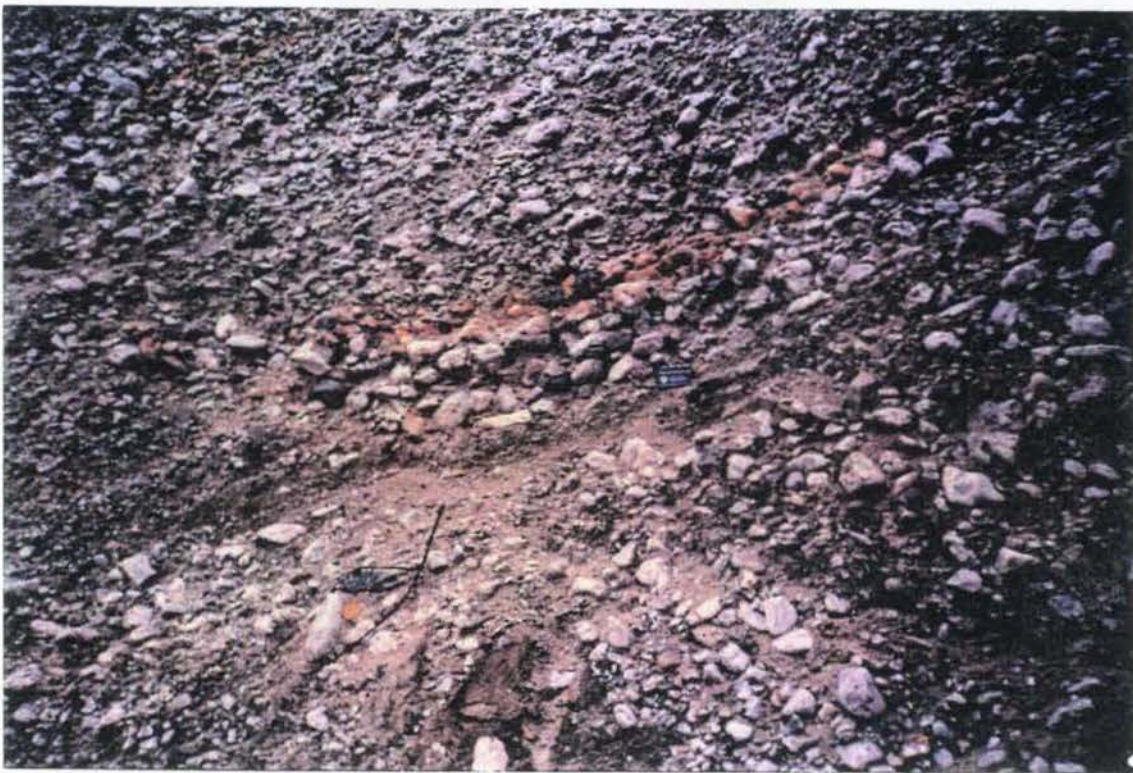
Figure 5: Cobble lag at the base of scour and fill facies. Openwork gravel layer at top of cobble lag is bright orange colored. Card at base of cobble lag (arrow) is 9 cm wide.
