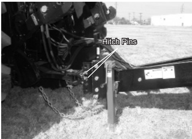
Figure C7 Adjust Hitch To Level Trailer
