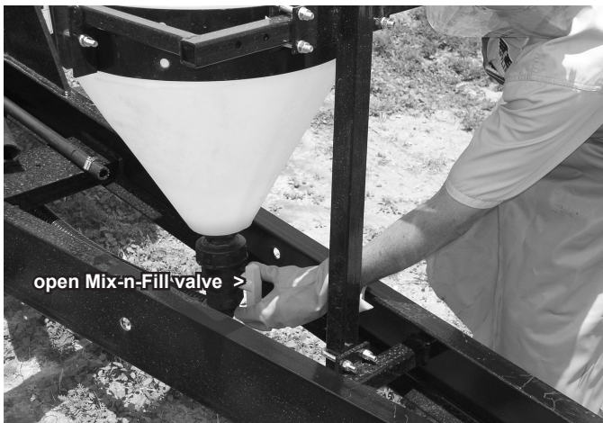
Figure B5 EP-1000 Chemical Induction
