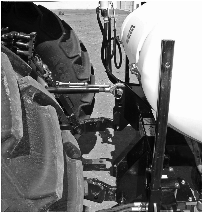
Figure A1 Mounting 3 point VSB to tractor
