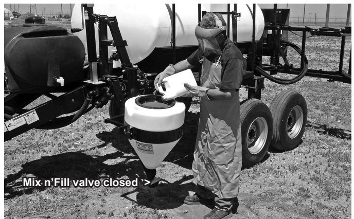
Figure B7 Adding Chemical To Mix-n-Fill Tank
