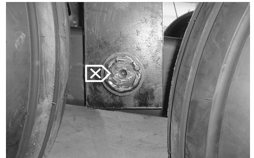
Walking Beam Pivot Grease every week
