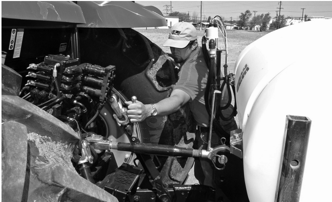
Figure B13 Adjusting Top Link To Level Boom
