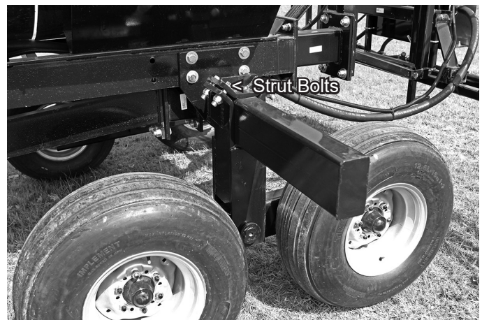
Figure C8 HCS Tandem Axle Adjustment
