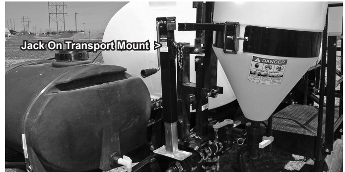
Figure A3 Jack Mounted For Transport
