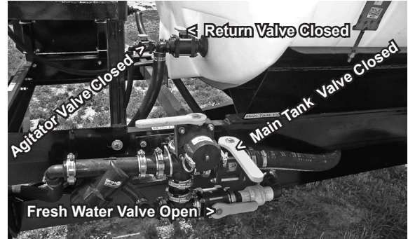
Figure B14 Valve Setting For Fresh Water Flush
