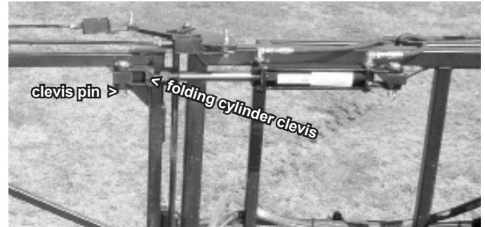
Figure C5 Adjusting Primary Wing
