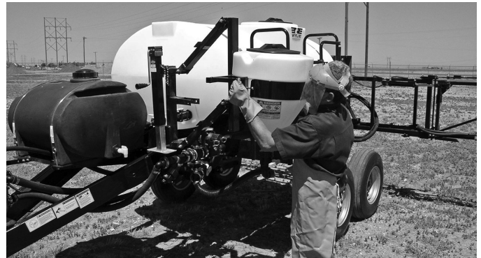
Figure B7 Lowering Mix-n-Fill Tank
